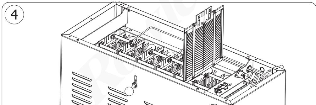
Step4: Take out the damaged heating element.
