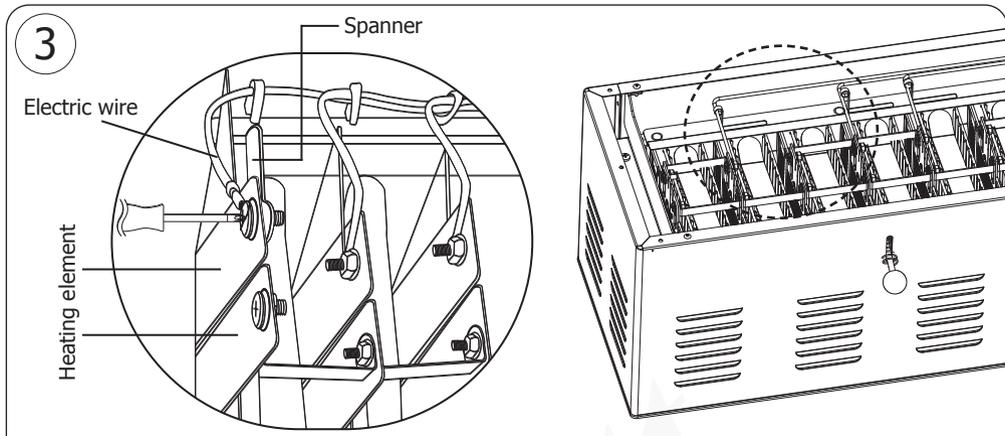
Step3: Lift the damaged heating element. Then use the spanner to hold the nut whilst using the screwdriver to loosen the screw, thus the heating element can be released.
