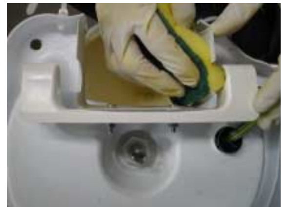
24. Reinstall stainless steel bottom removed at # 16 paying attention that its opening windows faces toward to the ice funnel area at # 5.
