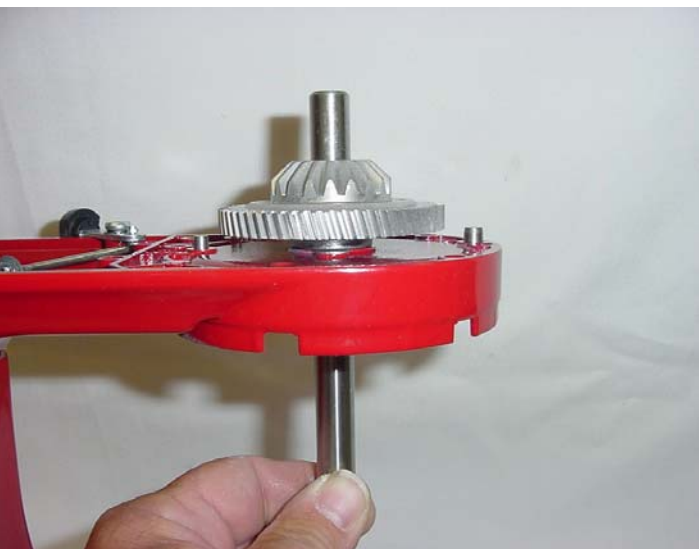
Fig. 54 Removal of vertical shaft from bottom cover.
