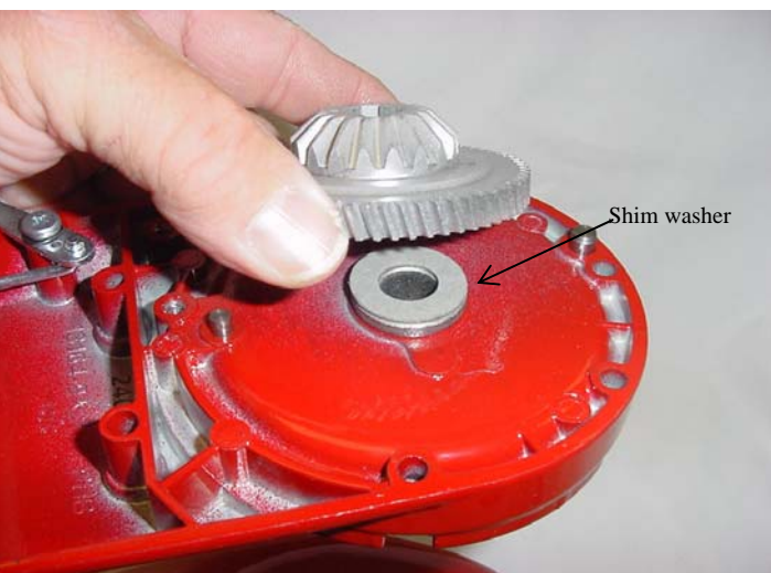
Fig. 55 Bevel center gear being lifted for inspection.
