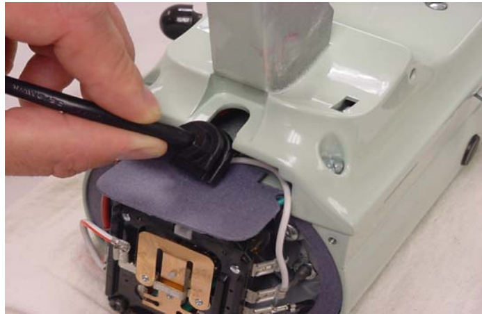
Fig. 8 Pull back on the molded strain relief to remove the power cord from the slot in the bottom cover.
