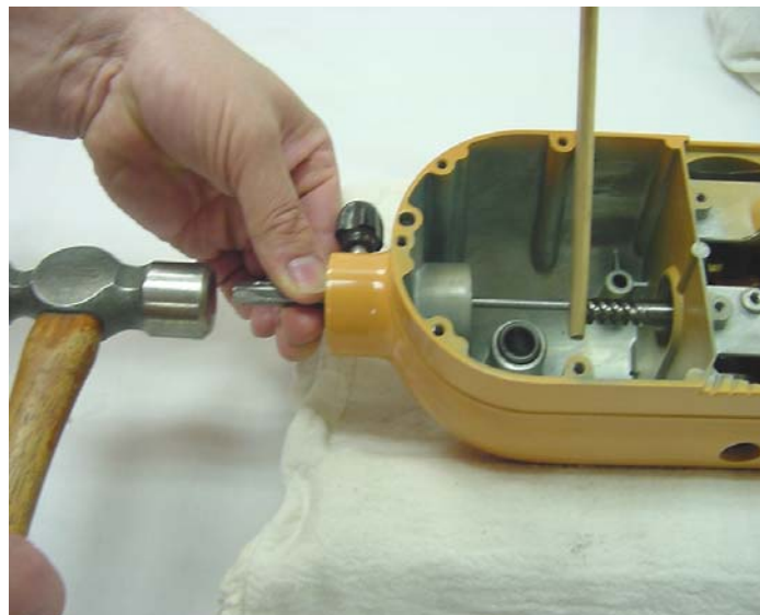
Fig. 30 A block of wood is used to protect the motor shaft when removing the armature.
