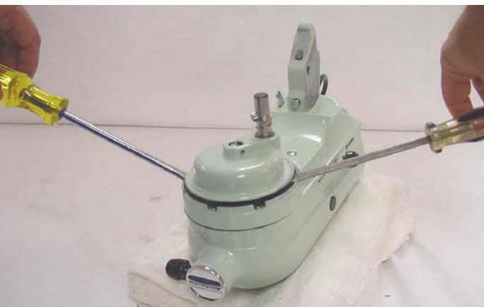
Fig. 7 Use two screwdrivers to pry the planetary off the shaft.
