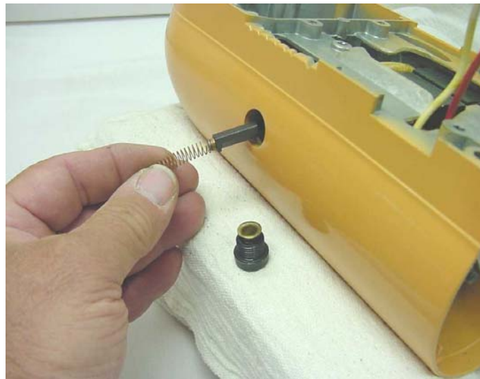
Fig. 29 the brush holder caps are loosened to access brushes for removal. Make sure to mark orientation.
