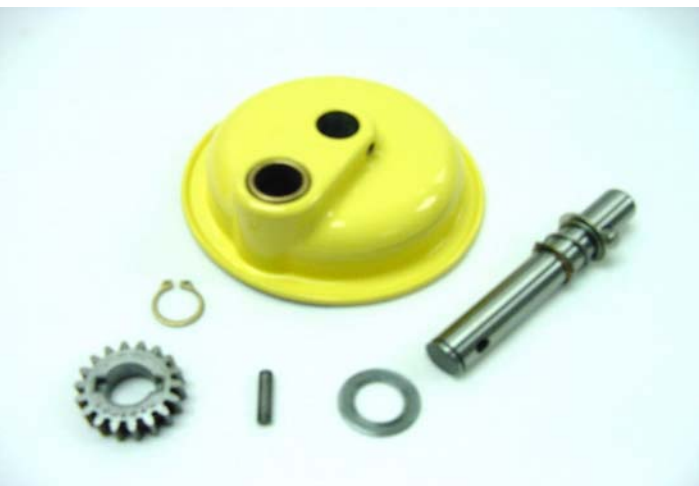
Fig. 66 The planetary components are shown disassembled.
