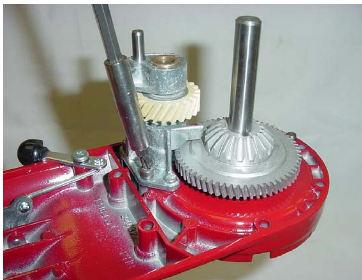
Fig. 52 Worm gear bracket bearing and pin assembly.
