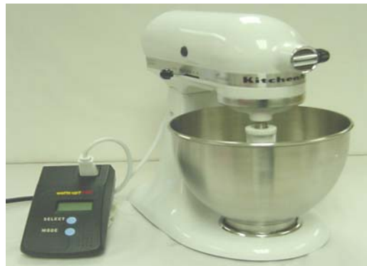
KitchenAid stand mixer shown with a digital wattmeter
