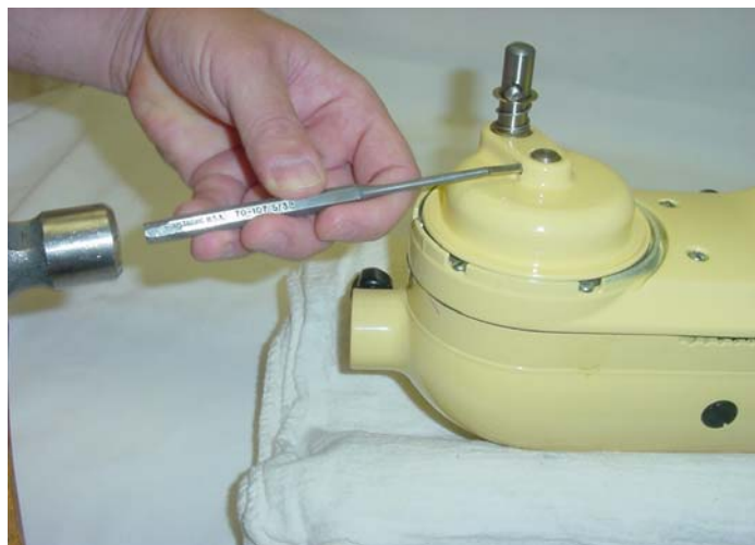
Fig. 68 Carefully drive the groove pin into the shaft of the planetary.
