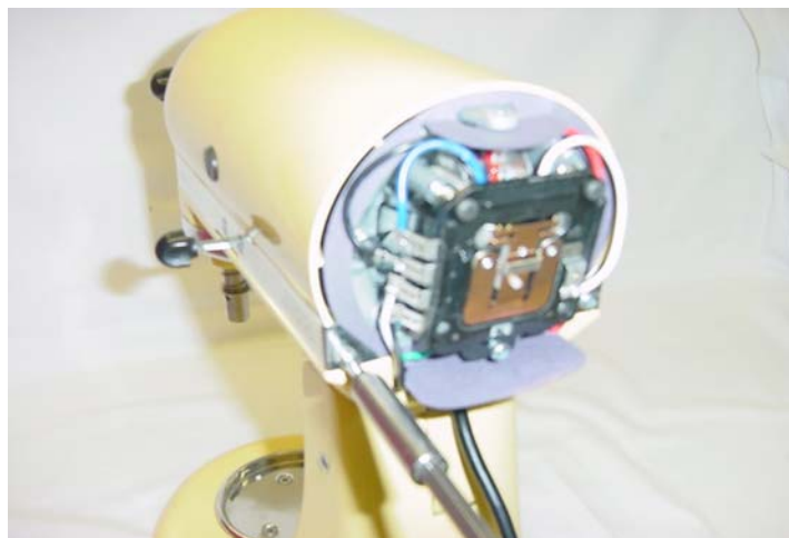
Fig. 81. Replace the trim band on the gearcase after speeds have been set.
