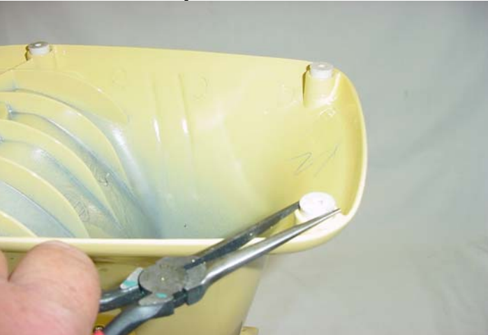
Fig. 71 The pedestal feet should be replaced on older mixers.
