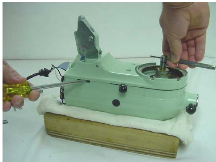
Fig. 12 While lifting up on the center shaft, use a screw driver to gently pry the bottom cover from the housing.
